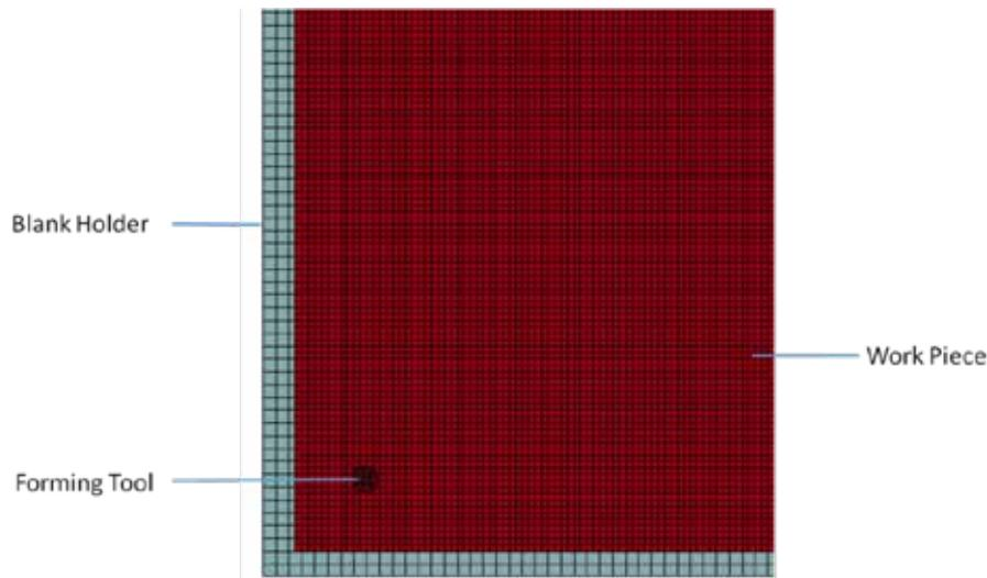
Fig. 3 The incremental sheet forming model (1/4 of the model): a sheet blank resting on a blank holder is gradually formed by a cylinder forming tool.
