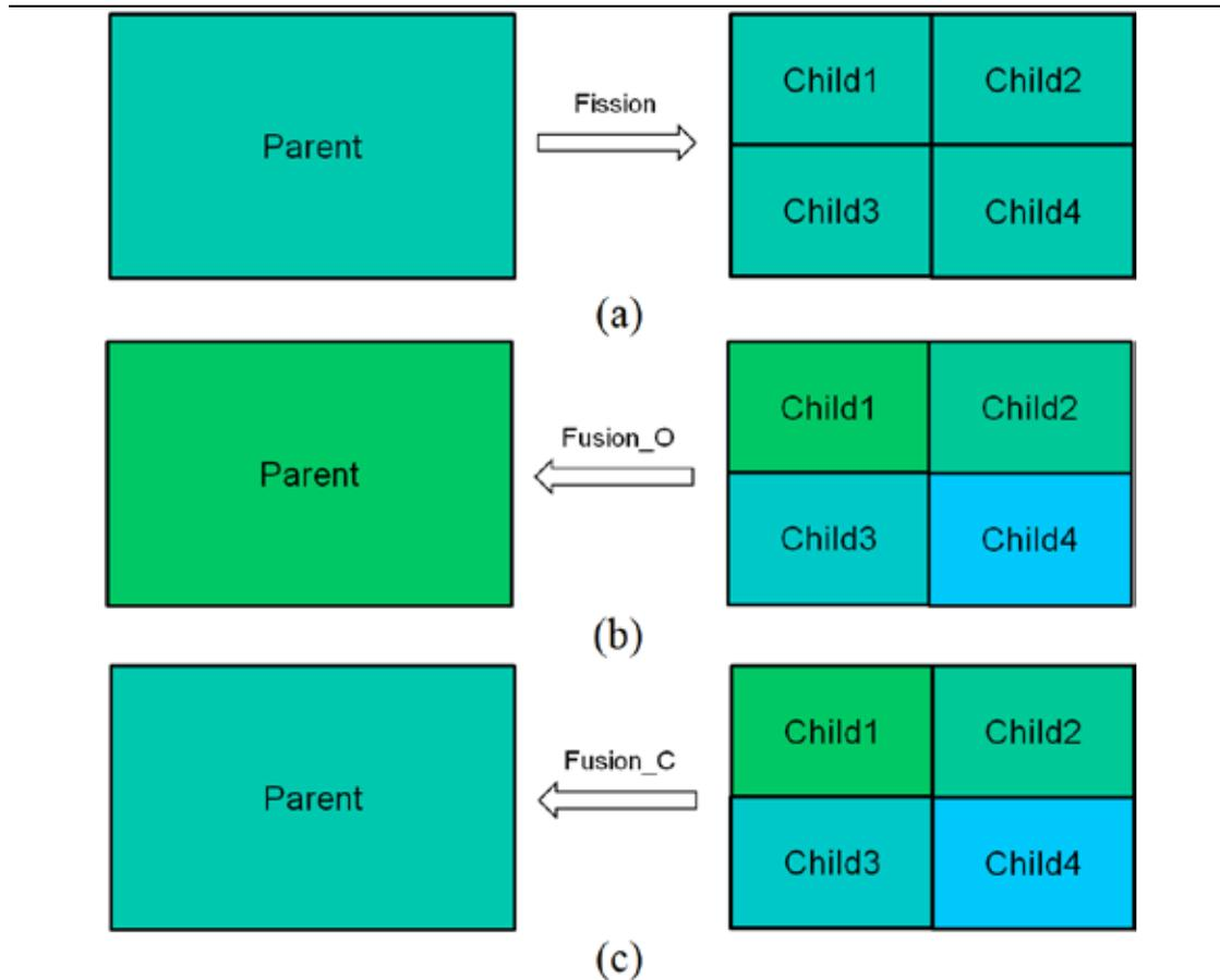
Fig 2: Property Inheritance in the Mesh Fission/Fusion Scheme: (a) Fission---All four child elements gets a complete copy of parent element's property; (b) Original Fusion Scheme---The parent element directly takes the property of child1, discarding the properties of the rest child elements; (c) Current Fusion Scheme---The parent element's property is treated as the average of those from the four child elements.
